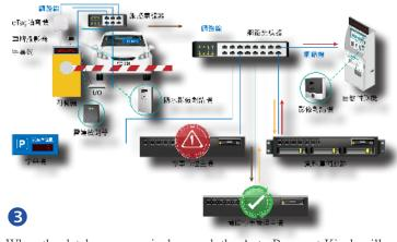
When the database server is damaged, the Auto Payment Kiosk will automatically read the relevant data from the parking management server.
