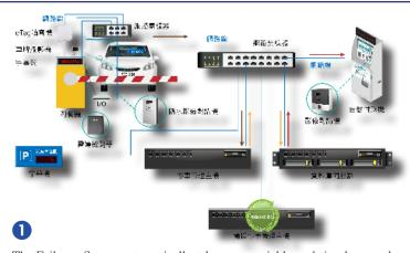
The Failover Server automatically takes over quickly and simultaneously downloads the latest data from the database server.
